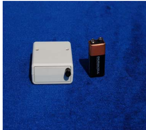
Radio transmitter and integral microphone
