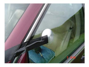
Wind Noise Microphone attached using double sided tape on a SUV and a saloon car.
